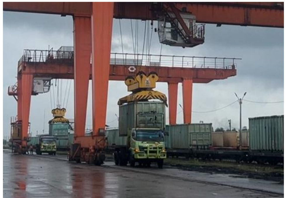
Figure 4. Container-to-Dump Truck Handling via Crane
